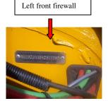
**SERIAL NUMBER LABEL** – A fireproof label shall be furnished showing the Vehicle Identification Number, and permanently affixed on the firewall in a position for maximum visibility and legibility (exact location to be approved). Letters and numerals shall be of the cut or embossed (metal) type. The serial letters and numerals should be at least one-fourth inch in height. (See picture for location).
