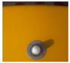
light shall meet SAE J1318 and J575 standards. Strobe light is to be Specialty Model 205 or equivalent. (See picture for approved light location.) Light shall be grounded to structural support.
