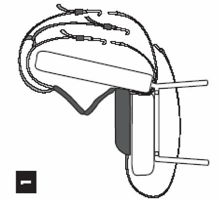
Place the STAR restraint on the bus seat. Place the three (gray, tan and black) cam wrap straps around the school bus seat back. Insert the short gray and tan straps connected to the rear of the STAR flexible seat base through the opening in the seat aushion (See Figure 1).
