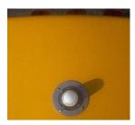
on position. The light shall meet SAE J1318 and J575 standards. Strobe light is to be Specialty Model 205 or equivalent. (See picture for approved light location.) Light shall be grounded to structural support.
