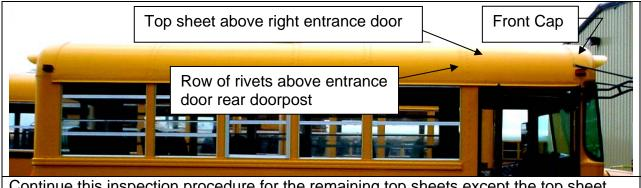
Continue this inspection procedure for the remaining top sheets except the top sheet above the right entrance door. This top sheet above the right entrance door, which attaches to the front cap, does not require inspection. Therefore do not measure the row of rivets above the entrance door rear doorpost; it is not part of the inspection procedure.
